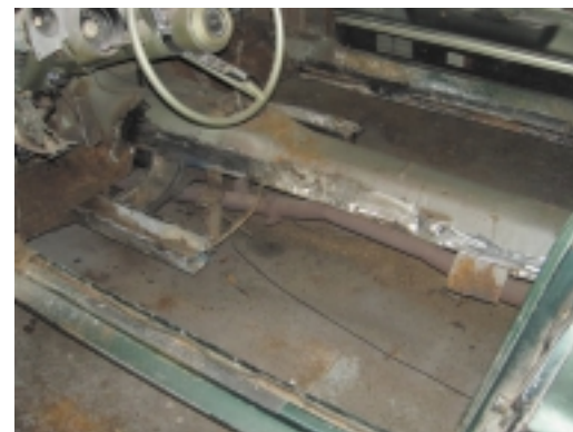
... except the floor panels which had perished. These were cut out and replaced. Kirk did this prior to removing the roof panel which ensured the rigidity of the car was maintained
